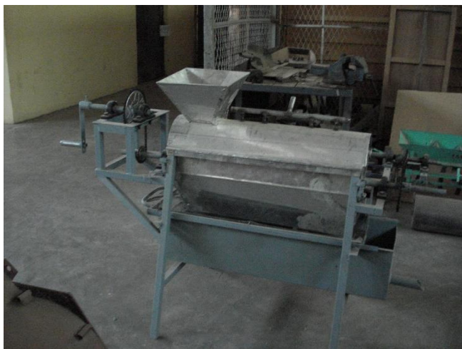
Figure 3. The final tomato extractor
