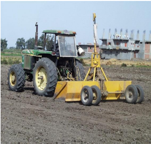
Figure 1. Laser land leveling
