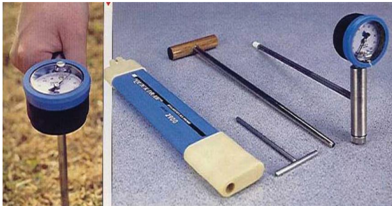
Figure 4. Tensiometer installed in the field
